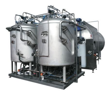
Designed for disinfection of biological waste and waste water before discharge into the sewer - the destruction of pathogenic microorganisms of I-IV hazard groups. Sterilization of effluents is carried out by heat treatment, varying the process time and heating temperature. Wastewater decontamination plants consist of:
